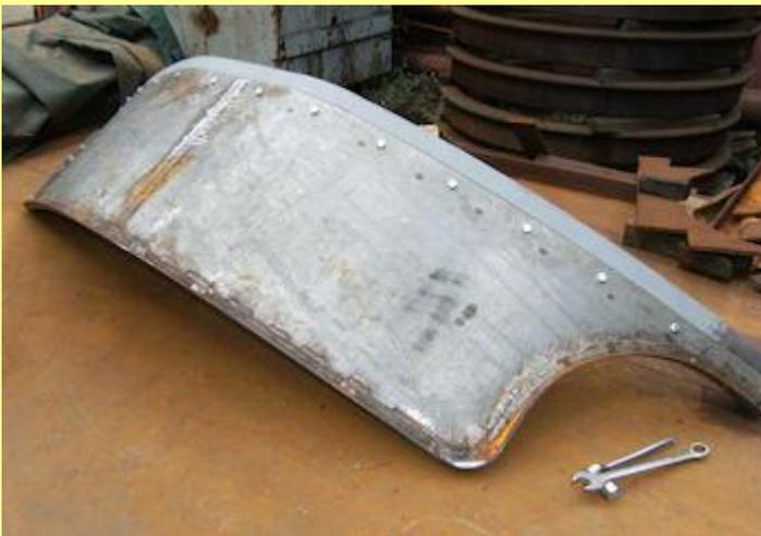
03/08/2013 Rear section of cab roof, prior to fitting.
