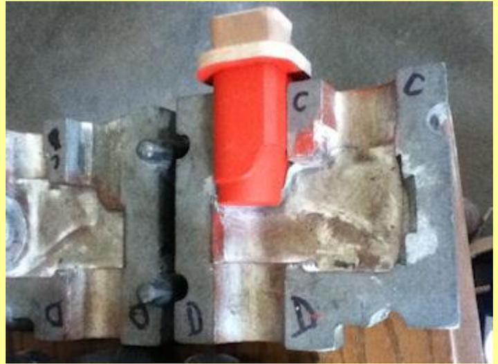
07/08/2013 - replacement core plug for the vacuum pump.
