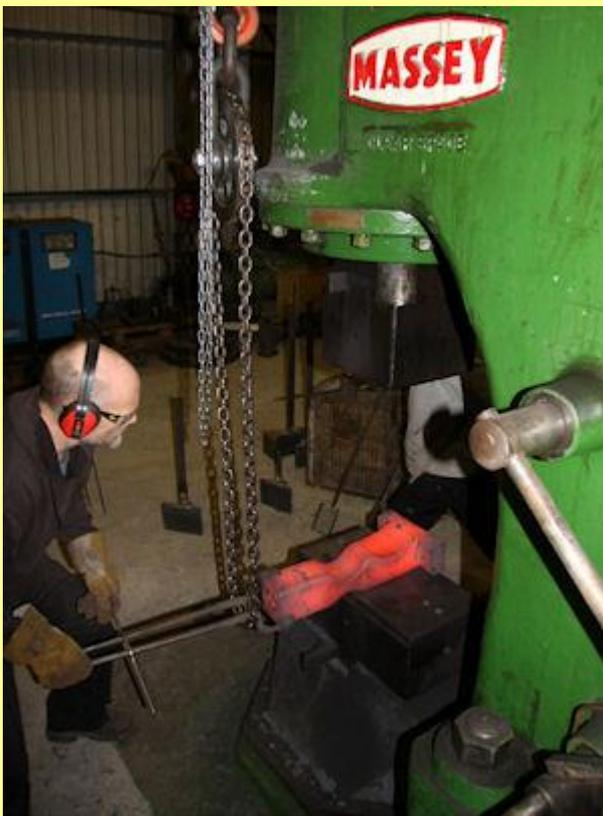
30/11/2013 - Forging begins - hot eccentric rod in place for the forging hammer to do its work.
