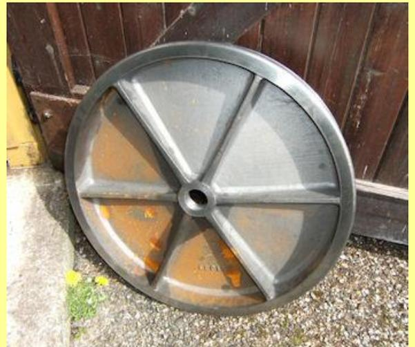
27/04/2013 - vacuum cylinder piston front view - machining complete.
