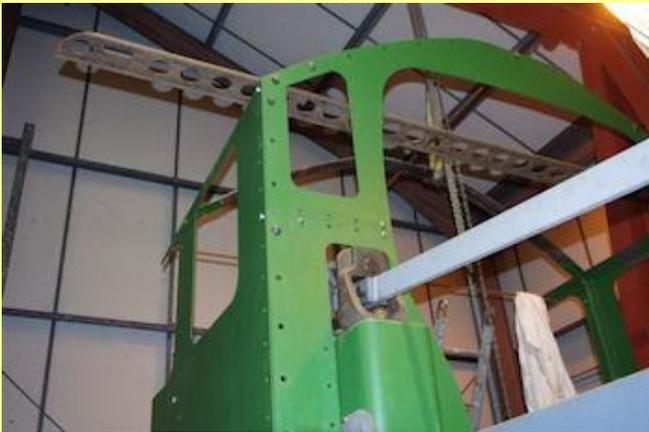
20/04/2013 - external view of front, right hand cab side bolted together before checking for its being square.
