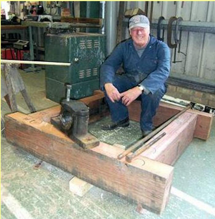
Terry Pattinson has completed the Gibbon frame and drilling the 22 mm holes in the frame. The 20 mm holes will be drilled next time. Discussions have taken place regarding fitting the axleboxes, ties and wear plates. Final completion is within sight.
