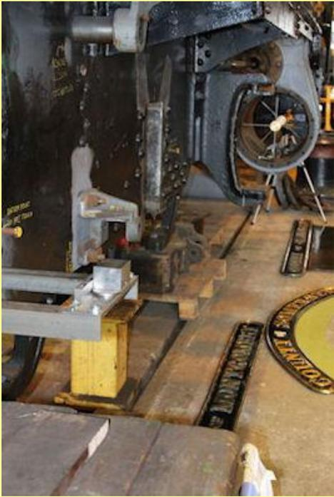
27/07/2013 - laser fitted in cylinder shining towards the square block on the jig fitted into the horn guide. (Terry McCarthy)
