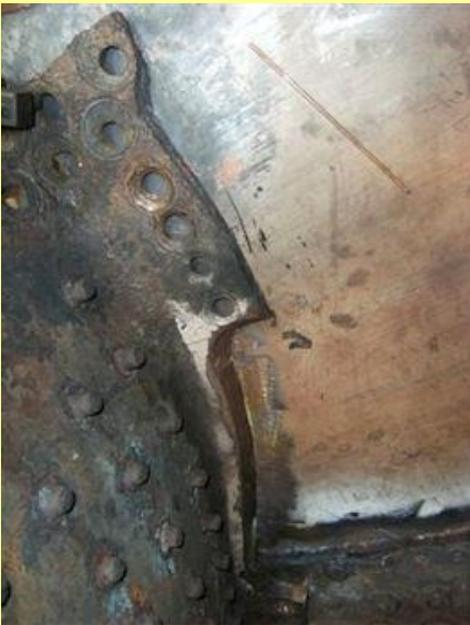
29/05/2013 - Lap repair to the firebox plates.
