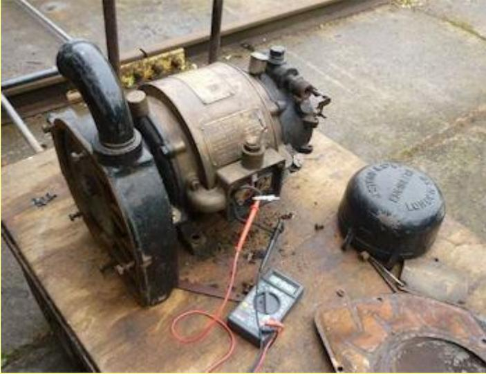
Acquisition of a steam generator to provide a battery charging capability for the on-board power for the TPWS/OTMR/speedometer system. It still looks expensive, particularly as our contact has discovered that the electrics do not work. This may act as an advantage as we would be able to purchase the non-electrical components and do a modern fit of a 24 V charging system.
