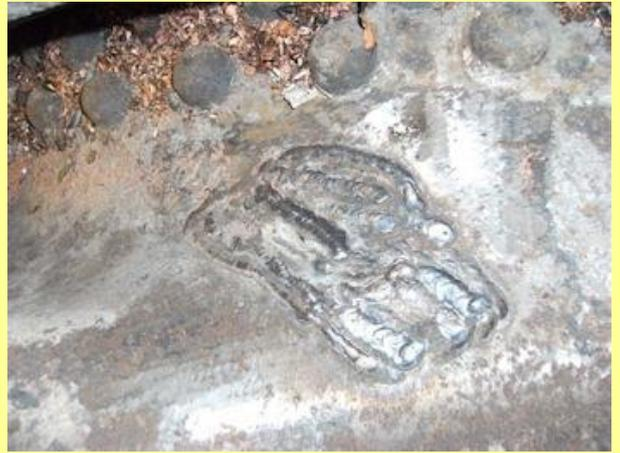
29/05/2013 - weld repair to firebox.
