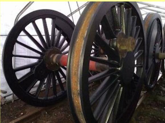
16/02/2013 - Progress on driving wheels - undercoat complete.
