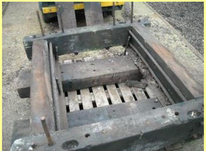
05/01/2013 - Following removal of the wheels the YAM is stripped to its basic wooden (oak) frame.
