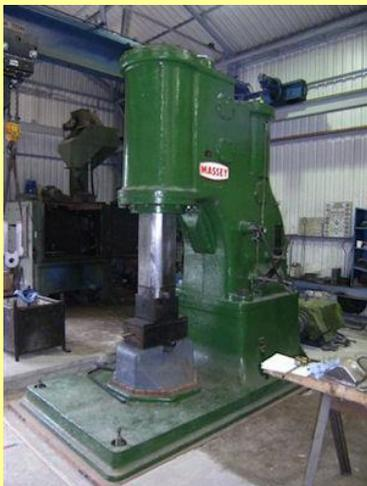
27/06/2013 - ASE's recently installed 8 ton hammer in the forging shop.
