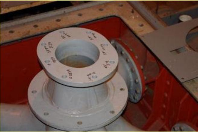
Fitting the 4 mudplates around the exhaust pipes in the exhaust box is now complete.
