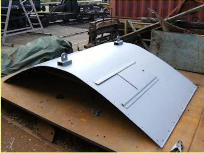
08/06/2013 - cab roof in primer. Sliding vents fitted and lifting lugs in position - latter will be removed once the cab roof is fully fitted.
