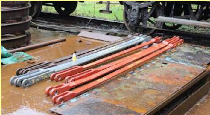
21/12/2013 - sets of locomotive and tender brake pull rods.
