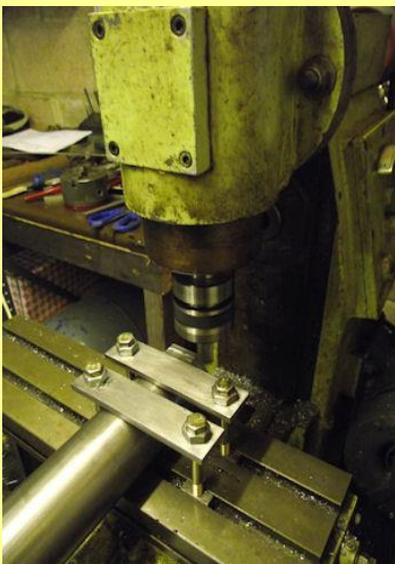
29/03/2013 - Drilling the distance tube.
