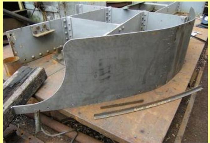
16/02/2013 - Rear cab roof section. being prepared for fitting.
