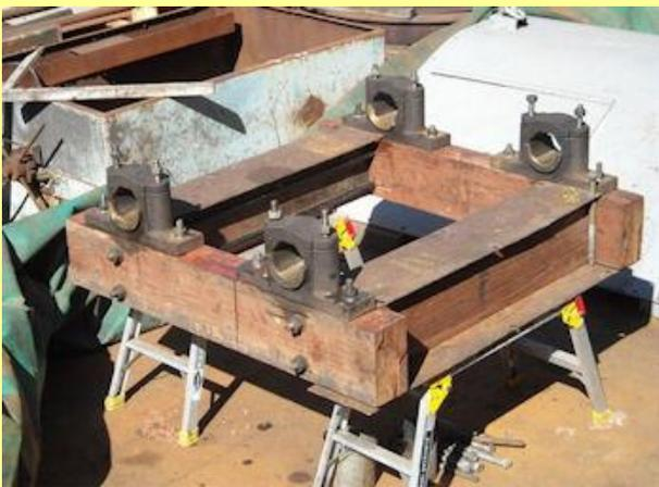
07/08/2013 - Yam frame bolted together with axle boxes fitted and bearing caps test fitted.
