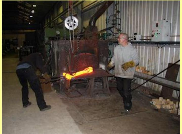
30/11/2013 - eccentric rod being withdrawn from the furnace.
