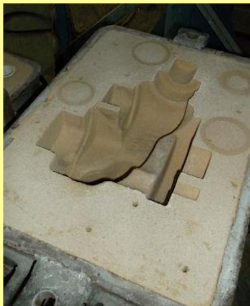
05/10/2013 - pattern for castings of the vacuum pump and its fittings.
