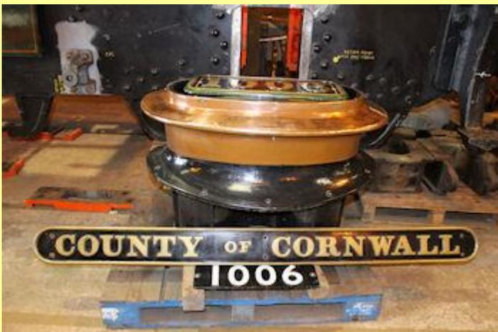
27/07/2013 - double chimney from scrapped County, 1006, donated to the Project in its early days shown with a left hand nameplate, cabside number plate and smoke box plate from the same locomotive - County of Cornwall scrapped in 1964 at Sharpness.
