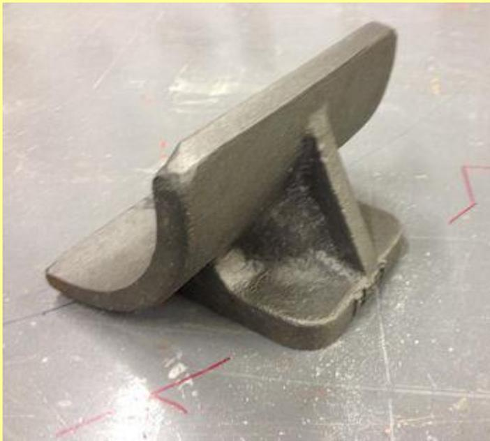
The steam fountain mount has been cast, and delivered to Crewe to be studded and welded to the firebox backhead.
