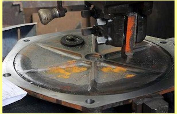
20/04/2013 - vacuum cylinder piston being machined.
