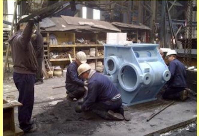
26/05/2013 - view of the poly-pattern produced for the 'Unknown Warrior' being prepared for casting. (Courtesy Unknown Warrior Project).
