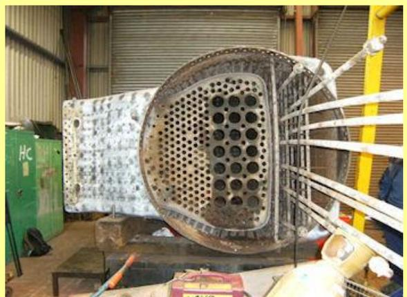
29/05/2013 - front tube plate of the inner firebox within the larger Belpaire outer firebox.
