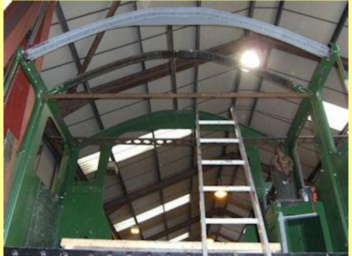
30/06/2013 - cab roof ribs fitted.
