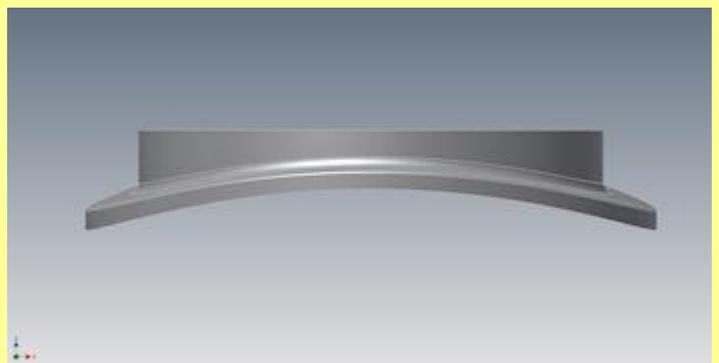
31/12/2013 - 3D image of the AutoCad file for the seating for the manhole and safety valve.
