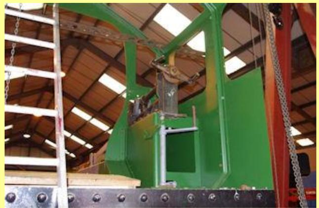
20/04/2013 - interior view of right hand side of cab - reversing screw and sanding control lever shown.
