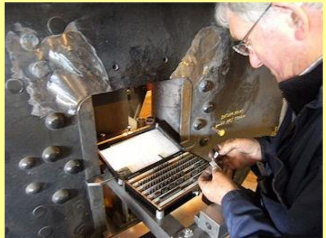
08/06/2013 - measuring horn guide alignment.
