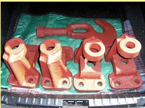
20/04/2013 - A boot full of cleaned and primed brake hanger brackets and a draw hook.
