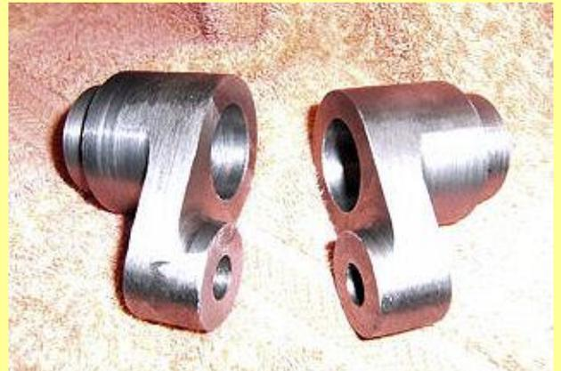
27/04/2013 - recently arrived and machined blow down valve components.
