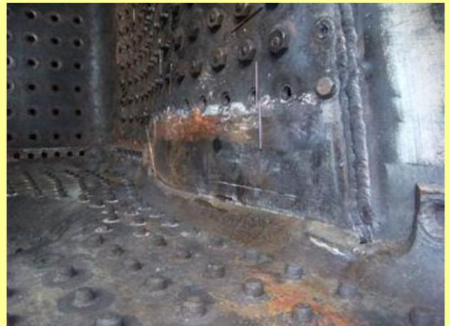
29/05/2013 - repairs to the firebox backplate.
