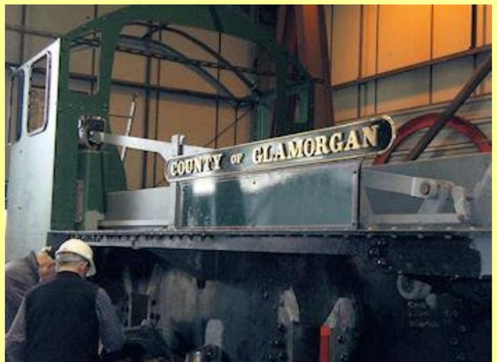
30/06/2013 - nameplate fitted, meanwhile work on measuring the axleboxes.
