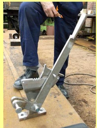
02/11/2013 - completed cylinder drain cock gear.
