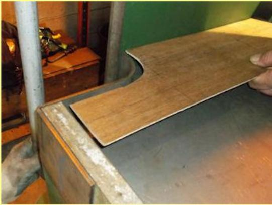
02/11/2013 - making and trial fitting the cab floor templates.
