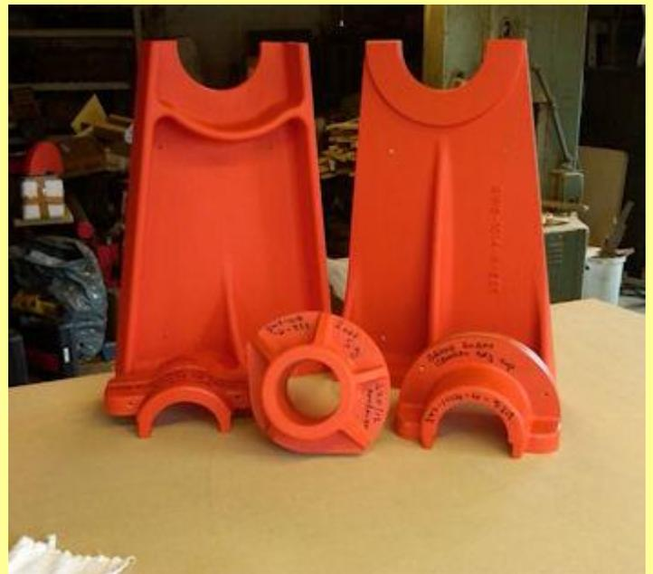
26/05/2013 - patterns for the tender brake shaft and accessories complete and ready for despatch to Stourbridge.
