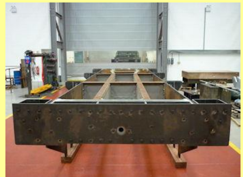
16/06/2014 - tender underframe fabrication completed. Derusting and priming to come before delivery to Didcot Railway Centre.
