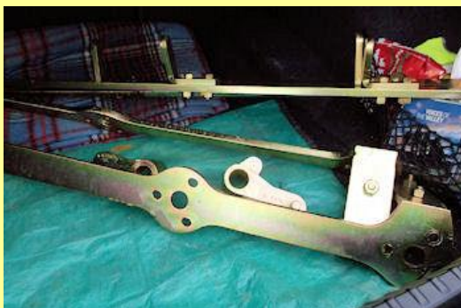
05/07/2014 - plated cylinder blow down cock gear.
