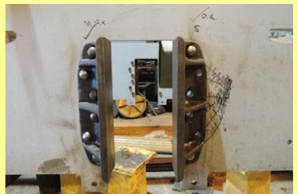
20/12/2014 - horns in place in the underframe.
