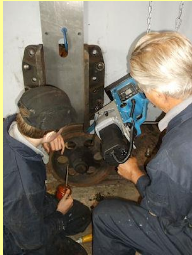
30/09/2014 - helped by the tender horn placement jig, drilling of the bolt/rivet holes to fix the horn guides in place is underway.
