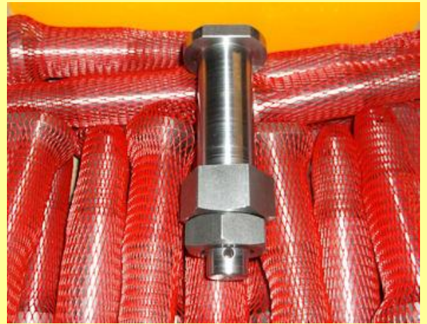
08/11/2014 - some of the beautifully finished brake gear pins.
