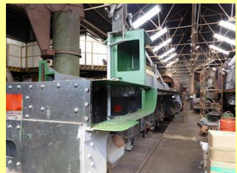
19/07/2014 - frames in lifting shop being readied for transfer to flat truck.
