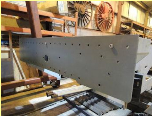
08/11/2014 - the rear buffering plate showing drilled holes.
