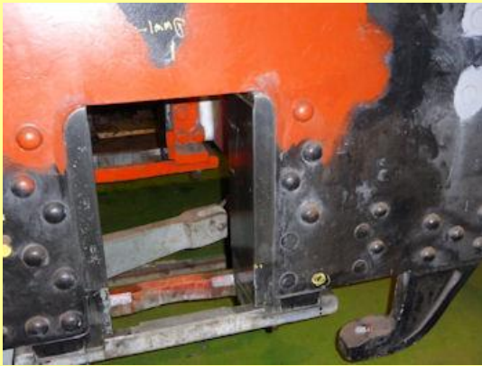
20/12/2014 - view of a horn block following alignment grinding to true.
