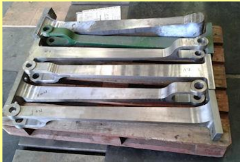
30/08/2014 - the new, unpainted eccentric rods as delivered to Didcot Railway Centre, with the master rod.
