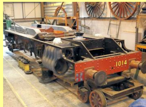
05-07-2014 - frames prepared for the move to Tyseley. The cab has been removed, along with other fittings and links. For the move, the frames will be removed from Number 4 road in the works at Didcot Railway Centre to the Lifting Shop, where it will be loaded onto a rail flat for the move to West Yard.
