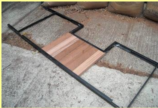
30/08/2014 - start of fitting timber into the cab floor frame.
