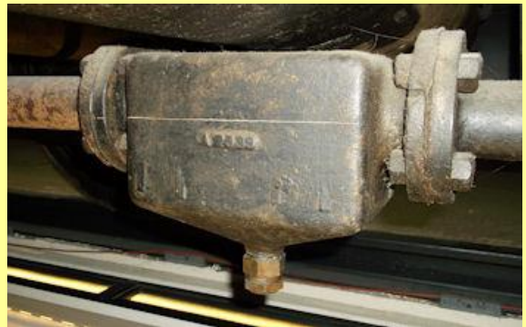
08/03/2014 - an example of the drip trap to be produced.
