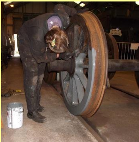
08/11/2014 - number 2 wheel set having been derusted is receiving a coat of primer.
