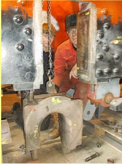
April 2014 - re-fitting axleboxes into horn guides.- preparing the lift.
