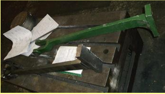
15/01/2014 - 'original' eccentric rod (green) alongside a new example at Arthur Stephenson Engineers.
