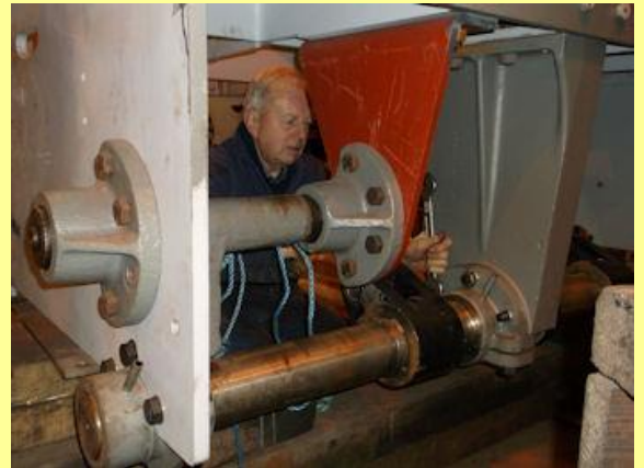
20/12/2014 - Gary trial fitting the brake cross shaft, cranks and bearings, plus water scoop linkages.
