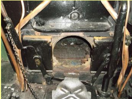
08/03/2014 - Fire hole doors, firebox hole and runners.
