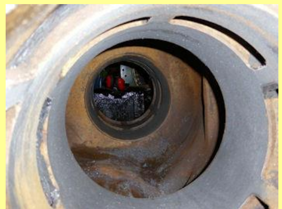
20/12/2014 - interior view of valve following boring.
