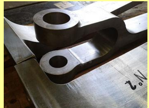
30/08/2014 - detail of the quality of engineering applied to eccentric rod.
