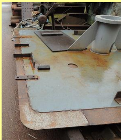
08/11/2014 - tender tank base now on steel slab, showing the steel corners and sides/ends tacked into position.
