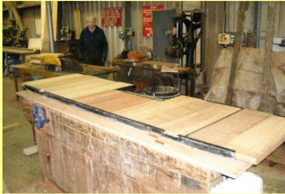
20/12/2014 - the completed cab floor, as fixed into the metal framework.
