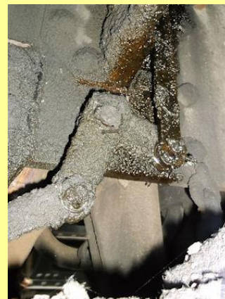
08/03/2014 - crank linking cab gear and rodding to the cylinder cock actuators.
