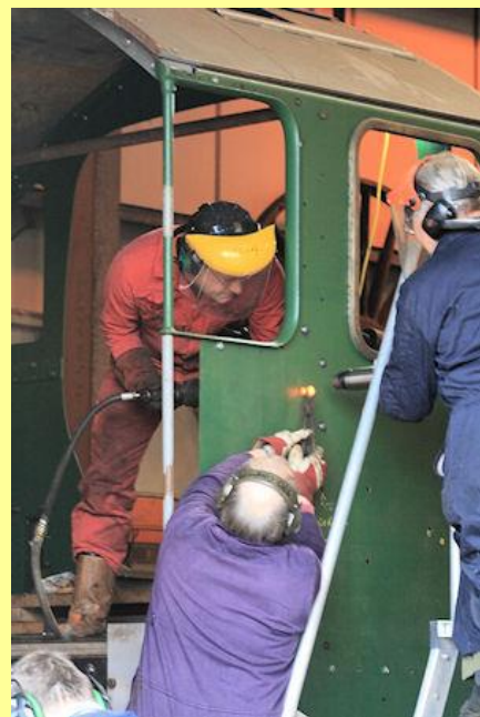
16 March 2014 - riveting team in action on the cab.
