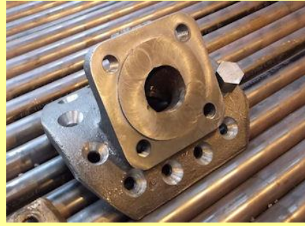
01/02/2014 - completed and machined steam fountain manifold.
