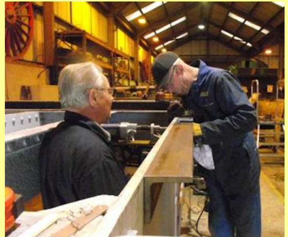
08/11/2014 - fitting the tank support angles to the tender main frames.
