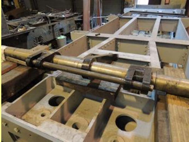
08/11/2014 - cranks tack welded to the brake cross shaft.
