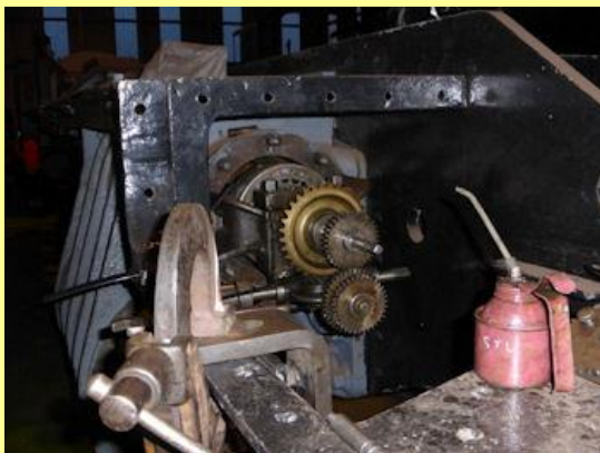
20/12/2014 - boring the right hand piston valves at Tyseley.
