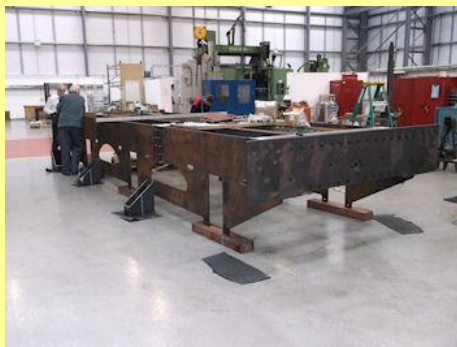
20/05/2014 - tender underframe being assembled.
