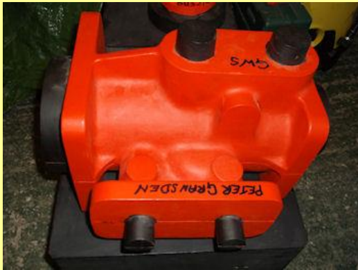
05-07-2014 - pattern for an exhaust steam injector.
