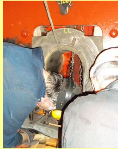
April 2014 - axlebox re-fitted into horn guide.
