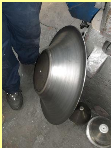
28/05/2015 - Chimney bell having been spun at Slough Metal Spinners, prior to delivery to Didcot Railway Centre.
