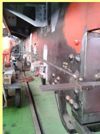
08/01/2015 - View of trammel bar in position between trailing and lead horns on left hand side of locomotive frame.
