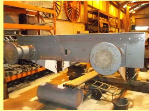
14/02/2015 - rear buffing plate fitted and awaiting riveting.
