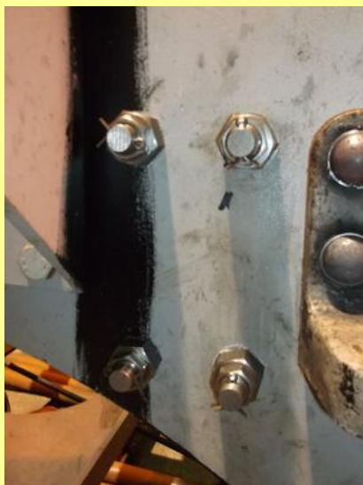
December 2015 - brake hanger brackets bolted into position.
