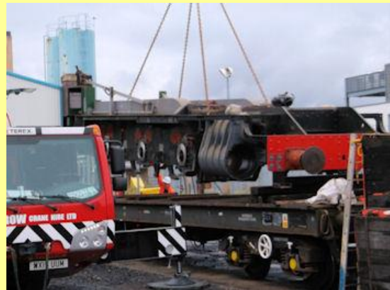
20/08/2015 - frames being lowered onto flat-bed wagon. (Mike Cooper)
