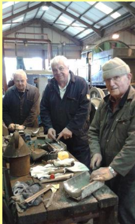
02/05/2015 - the Three Amigos scraping tender axle bearings.
