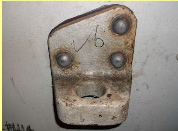
24/10/2015 - spring hanger bracket riveted in place on underframe.
