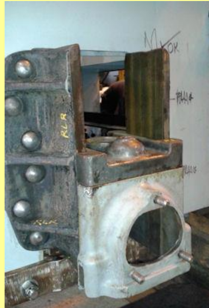
03/09/2015 - Axleboxes as received from Geoff Parker's works.
