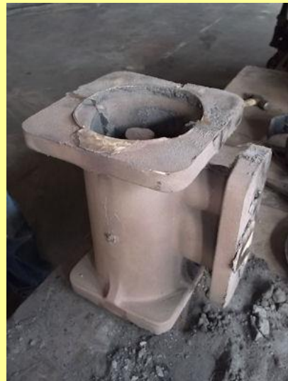
28/02/2015 - finished rough bronze casting of the exhaust steam injector body, removed from the mould box and yet to be cleaned up with a die grinder.
