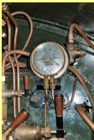
10/10/2015 - Vacuum Release Cocks - as fitted to another locomotive.
