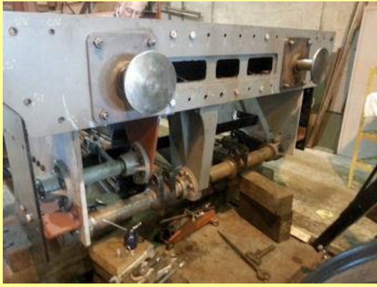
03-09-2015 - view of inner buffers and installed brake cross shaft.
