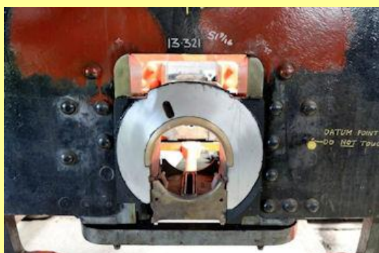
20/08/2015 - Close-up of machined and fitted bearings as fixed and trued on the main frames at Tyseley. (Frank Dumbleton)
