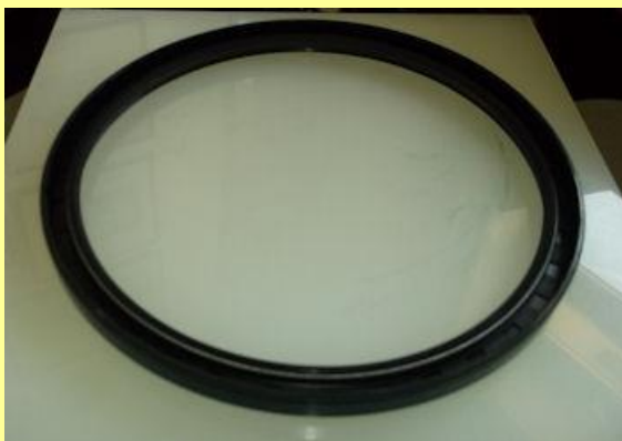
02/05/2015 - An improved axlebox oil seal arrangement is being developed, intended to replace the Helvetica leather on an elm carrier system, dating from the 1920s. This proposes to use a modern oil seal on a polypropylene carrier.
