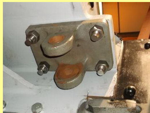
December 2015 - rear brake hanger bracket bolted into position.
