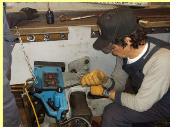
04/07/2015 - George drilling holes in the tender underframe for the Spring Hanger Brackets..
