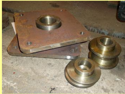
02/05/2015 - components of the inner buffing plates prior to fitting.
