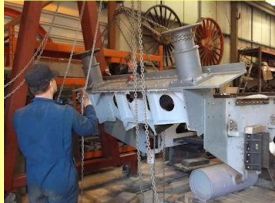
Replacement of the rear dragbox following the necessary drilling and riveting.
