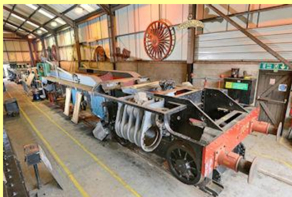
10/10/2015 - locomotive frames relocated on No. 4 road in the DRC Locomotive Works. Note the locomotive frames are supported at the front by the bogie, while to the rear are the tender frames.
