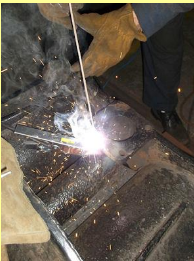
December 2015 - Gary undertaking welding repairs to the chimney blower flange.
