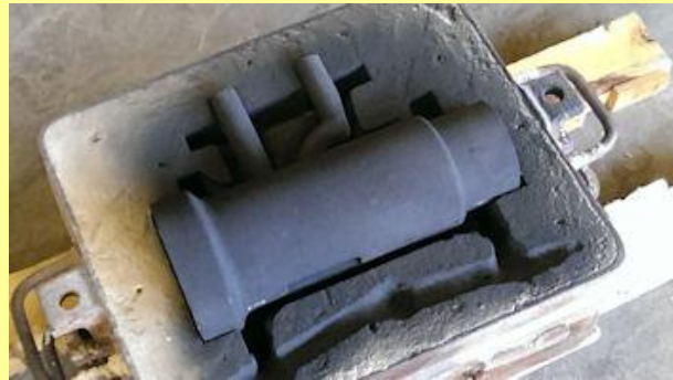
28/02/2015 - bottom half of the mould box showing the pattern removed and cores placed inside the mould to produce the cavities inside the casting. Hollow risers are added in various places to allow the molten metal (bronze in this case) to flow into all parts of the casting mould.
