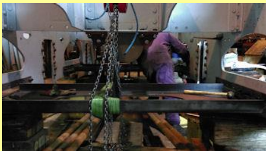
02/05/2015 - Cross stay plates have been fitted but the support angles remain to be riveted..
