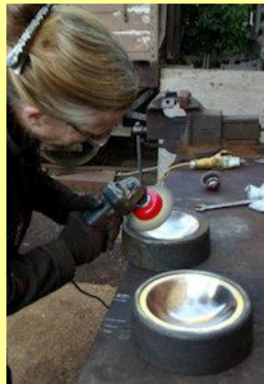
10/10/2015 - LaDonna working on the bogie bearing pads.
