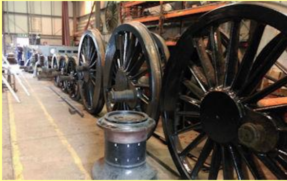
22/08/2015 - workshop view shewing 1014's driving wheels, tender wheels and to rear tender frames. (Mike Cooper)
