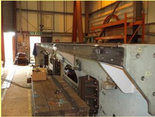
03-09-2015 - Valences set-up on frame angles.
