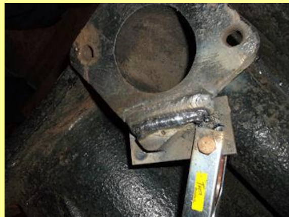
December 2015 - welding repair completed - now for fettling.
