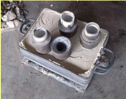
28/02/15 - a complete mould box showing the hollow feeds which also act as expansion risers for the LG4 grade casting bronze.
