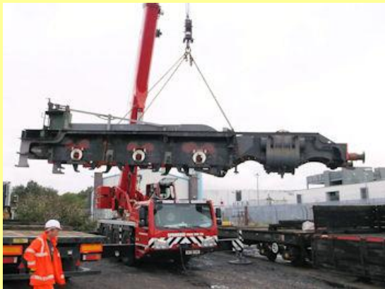
20/08/2015 - frames suspended having been lifted from lorry before being loaded on to flat-bed wagon for removal into Didcot Railway Centre. (Mike Cooper)
