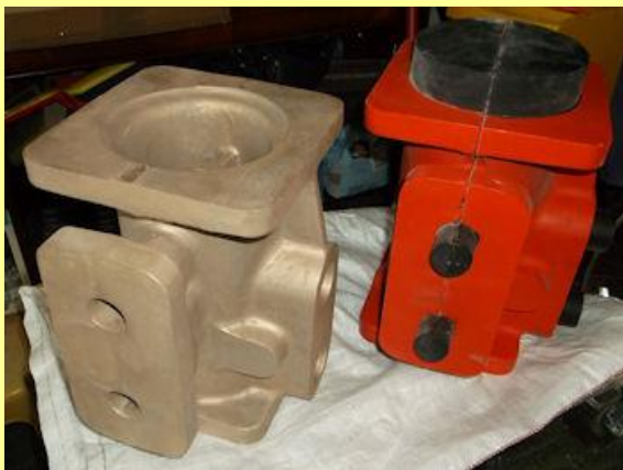
02/05/2015 - exhaust injector pattern (red) and casting.
