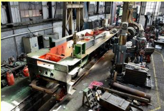
22/08/2015 - frames in lifting shop having been lifted off flat-bed wagon and lowered onto yam. (Frank Dumbleton)
