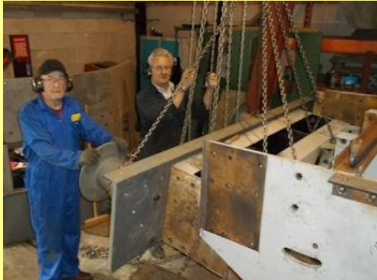
Removal of the rear dragbox in preparation for drilling the holes required
