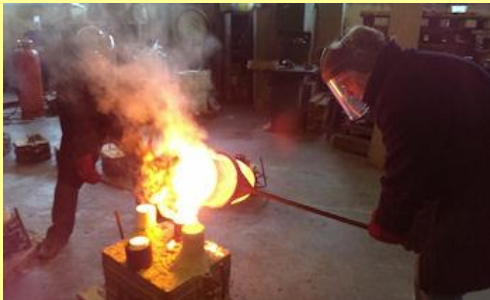
28/02/2015 - pouring the liquid bronze from the crucible into the mould box..
