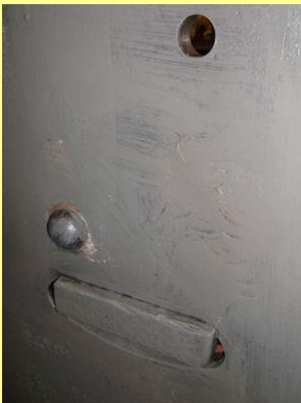
04/07/2015 - holes in process of being drilled for Spring Hanger Brackets..
