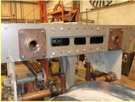
04/07/2015 - Front drag beam showing position of inner buffers.
