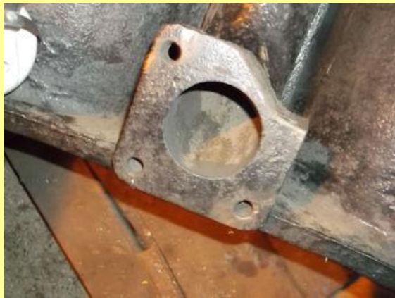
10/10/2015 - repair to the blower flange of the chimney.
