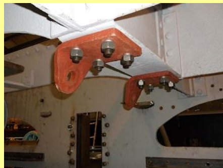
02/05/2015 - Various items of the water scoop gear await fitting to the brackets.
