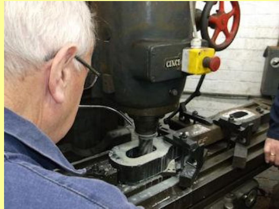
04/07/2015 - Gary machining drag links, i.e. the locomotive-tender coupling arrangement.
