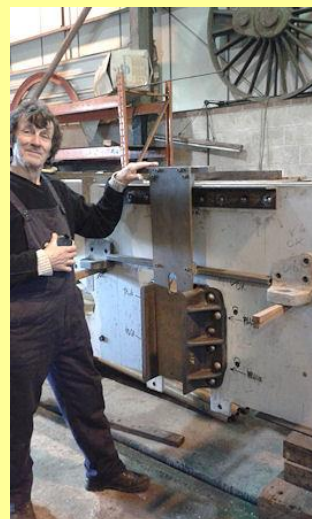
02/05/2015 - George's jig to fit the spring hanger brackets.
